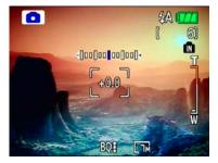
2. Use the **Left/Right** to adjust the exposure value for the picture. The range is from EV -2.0 to EV+2.0 (steps of 0.3).
